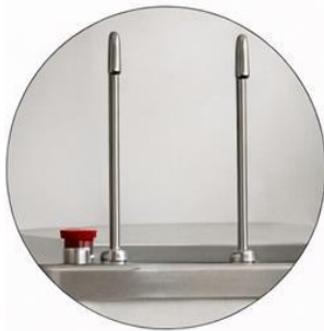
Bottle Filling Pipes Pipa Pengisian Botol
